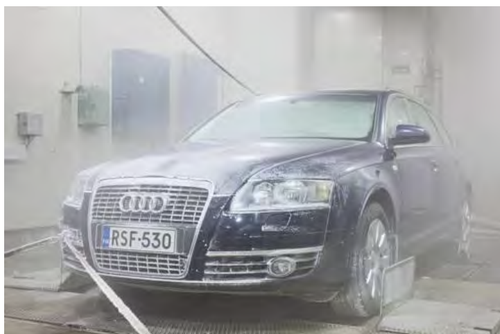
Figure. Testing of cold properties with diesel cars in a climate chamber..
