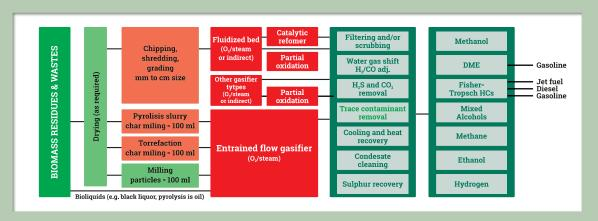
At present, only one advanced biofuel plant is in operation, the Enerkem plant in Edmonton, Canada that produces methanol or ethanol from assorted wastes (RDF) at a nominal capacity scale of 24,000 toe/year (toe, tonnes of oil equivalents). Up to 2018, also the GoBiGas plant in Gothenburg Sweden was in operation, producing bio-methane from forest residue pellets up to a nominal capacity of 14,000 toe/year, but was closed for economic reasons (lower than expected energy prices).
